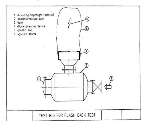
APPENDIX 3 - Schematic Plan of the Test Plant for High Velocity Valves (endurance burning test only)
